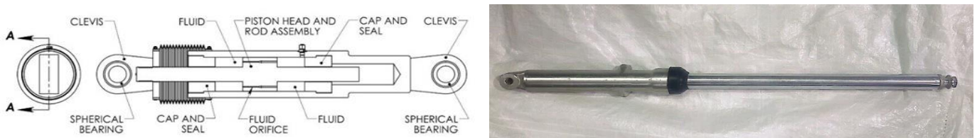
Fig. 2. Schematic representation of the viscous damper and its components
