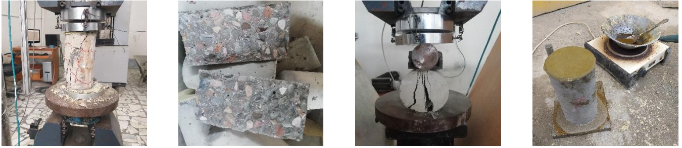
Fig. 5. Testing for the compressive and tensile strengths concrete
