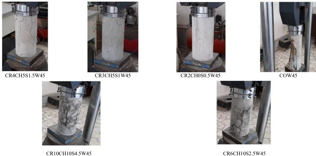
Fig. 6. Crack patterns and propagation in SCC samples
