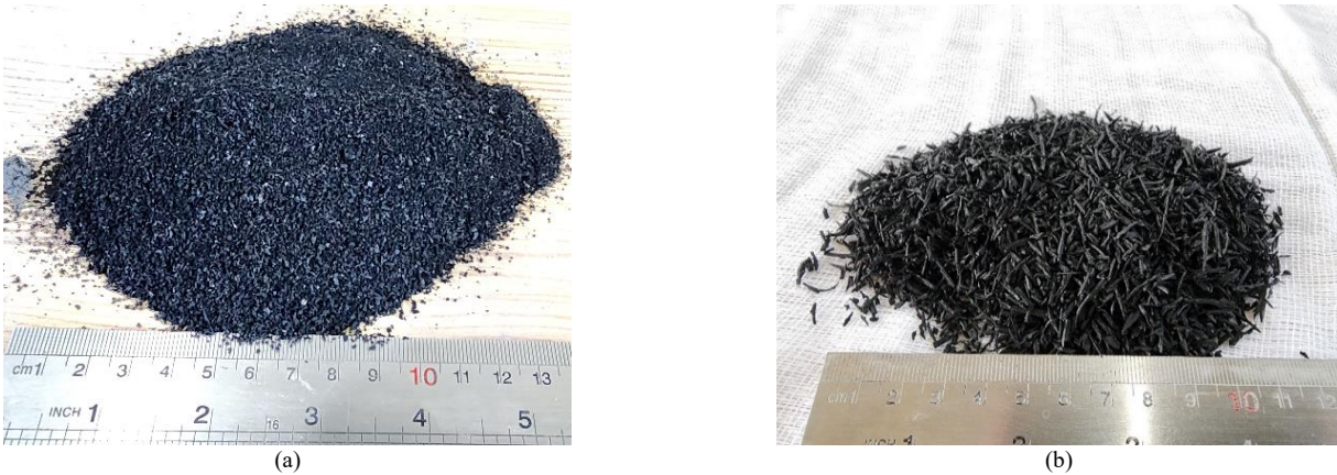
Fig. 1. Recycled tire-derived rubber aggregates used in this study: (a) rubber powder (0.5–2 mm) produced through cryogenic grinding; (b) rubber chips (2–5 mm) obtained from ELT shredding.
